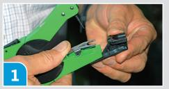
IMPORTANT: Remove/slide black insert out of female jaw.
