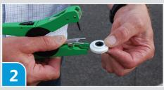
To load, depress spring clip and insert electronic tag, holding raised area between thumb and forefinger.
