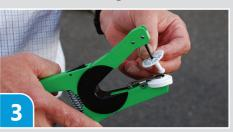
Slip male tag completely onto applicator pin.
